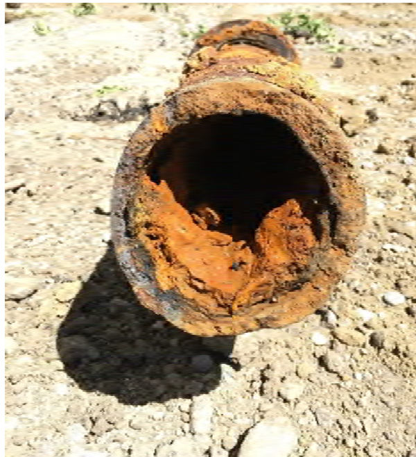
Figure 3.10: Typical Cast Iron Pipe Section
